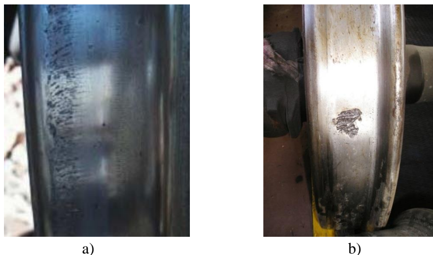
Figure 25.2. RCF damage of railway wheel: a – shallow; b – subsurface
