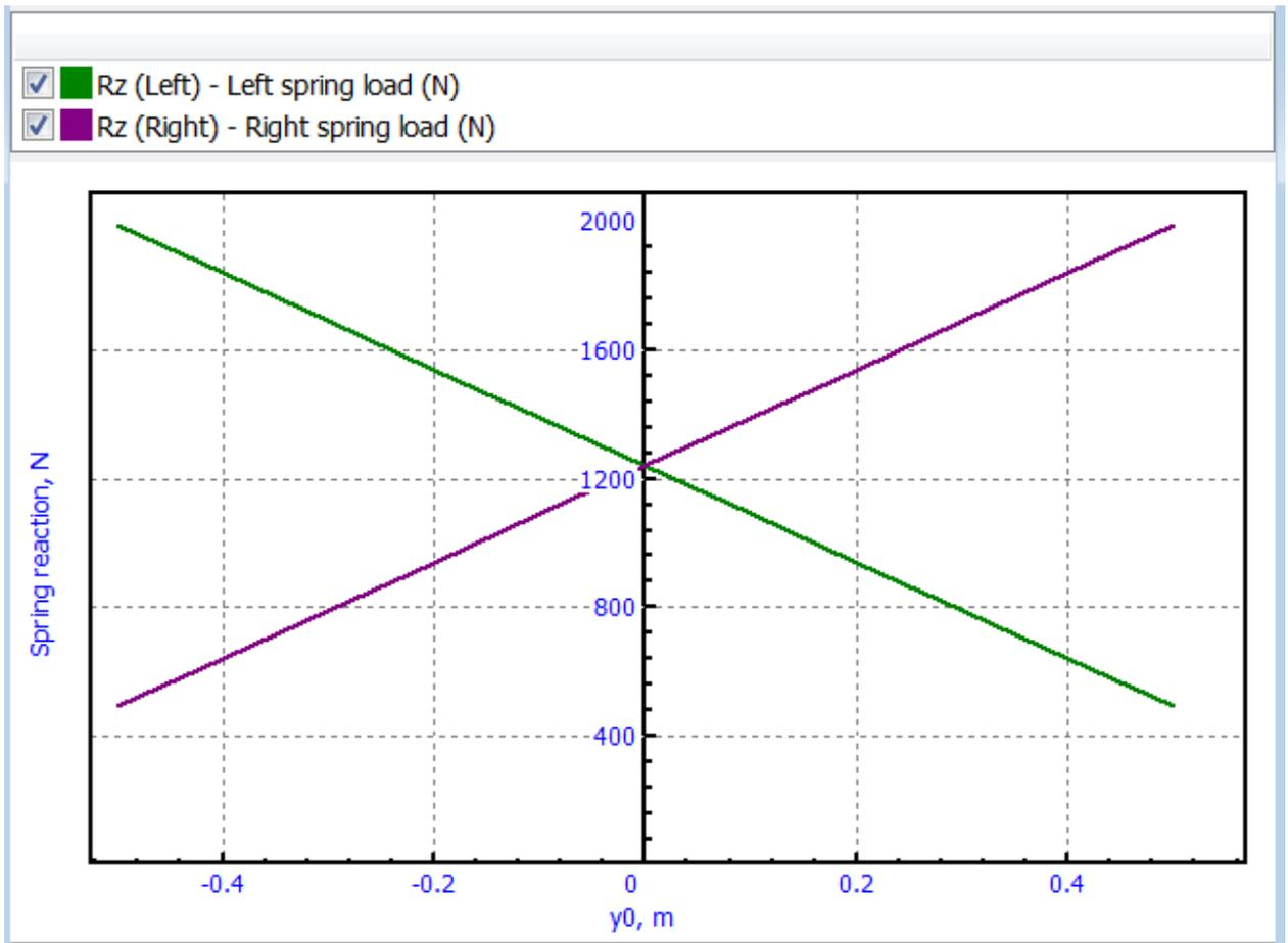
Figure 4.181. Static spring forces versus coordinate of load application
