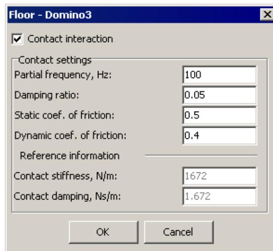
Figure 4.118. Parameters of contact interaction between two bodies
