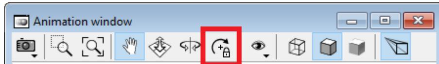
Figure 4.69. Fixation of the rotation center
