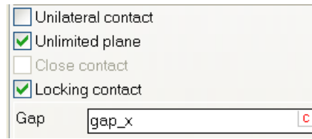
Figure 3.240. The locking mode of bilateral contact
