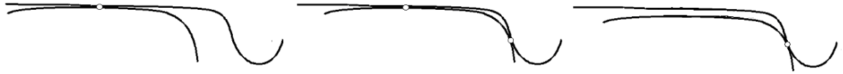
Figure 8.89. Types of contact for a pair of profiles allowing two-point contact: one-point contact, two-point contact and creeping up
