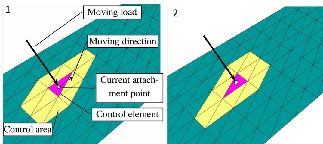
Figure 21.3. Control area for fast determination of the attachment point.
