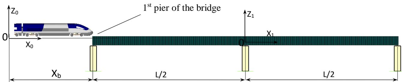
Figure 21.9. Position of **Bridge** subsystem in the railway track.
