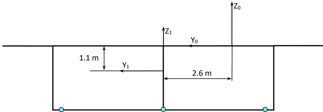
Figure 21.10. Bridge cross section and position of the local frame of reference.
