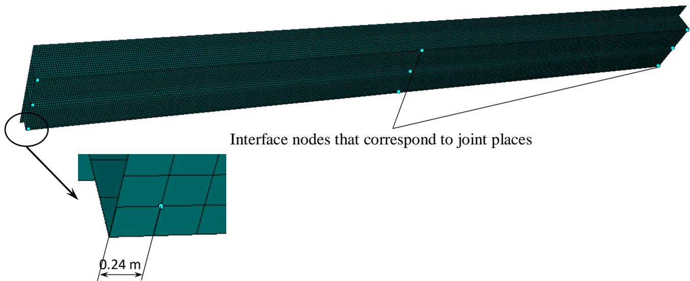
Figure 21.7. Interface nodes of flexible subsystem Bridge.
