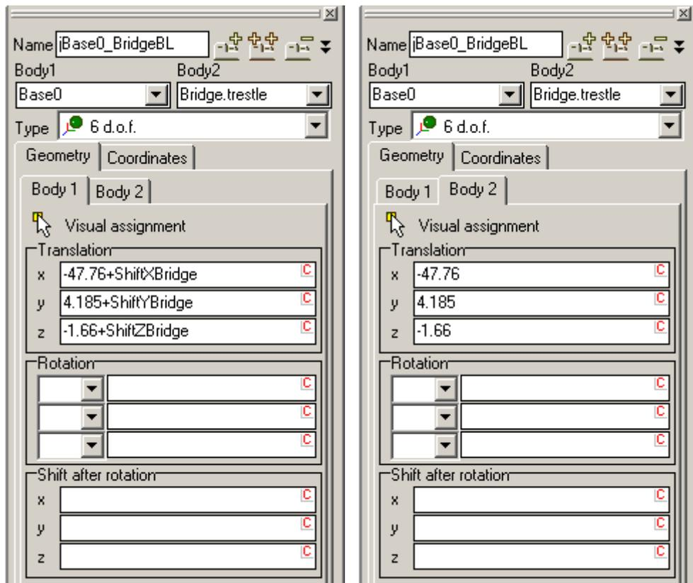
Figure 21.13. Coordinates of the joint point of the left joint on the 1st pier in the SC0 (left) and the local frame of reference of the bridge (right).
