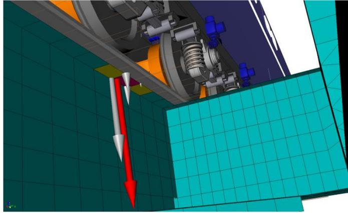
Figure 21.17. Vehicle-bridge interaction force and its reduction to nodal forces.
