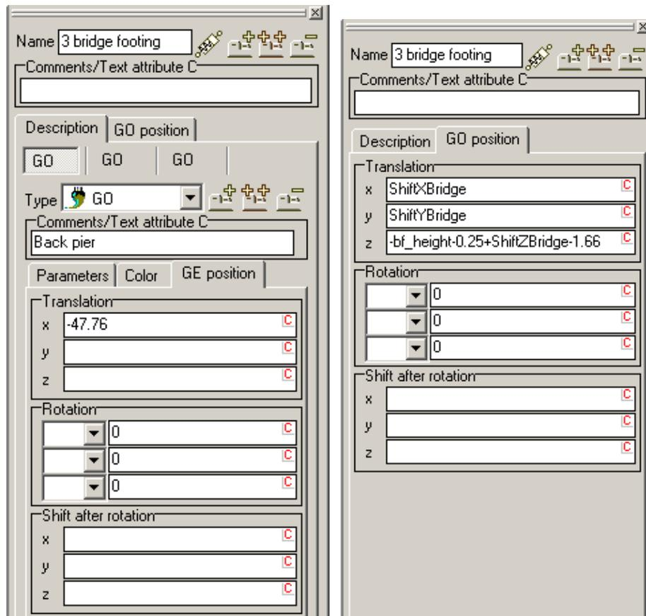
Figure 21.12. Position of the graphical object of the 1st pier (left) and position of **3 bridge footing** graphical object assigned to the scene (right).
