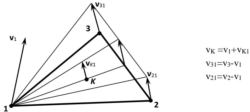
Figure 21.4. On calculation of velocity of an arbitrary point.
