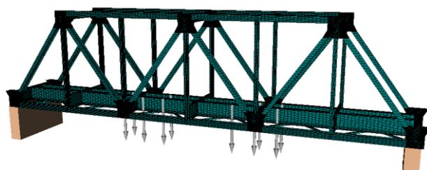
3. The obtained wheel-to-rail forces are applied to the correspondent points on the bridge.
