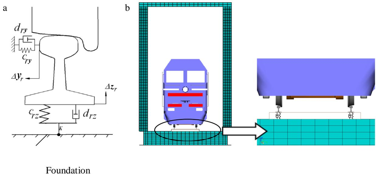
Figure 21.1. (a) rail as a massless force element; (b) visco-elastic foundation including bridge.
