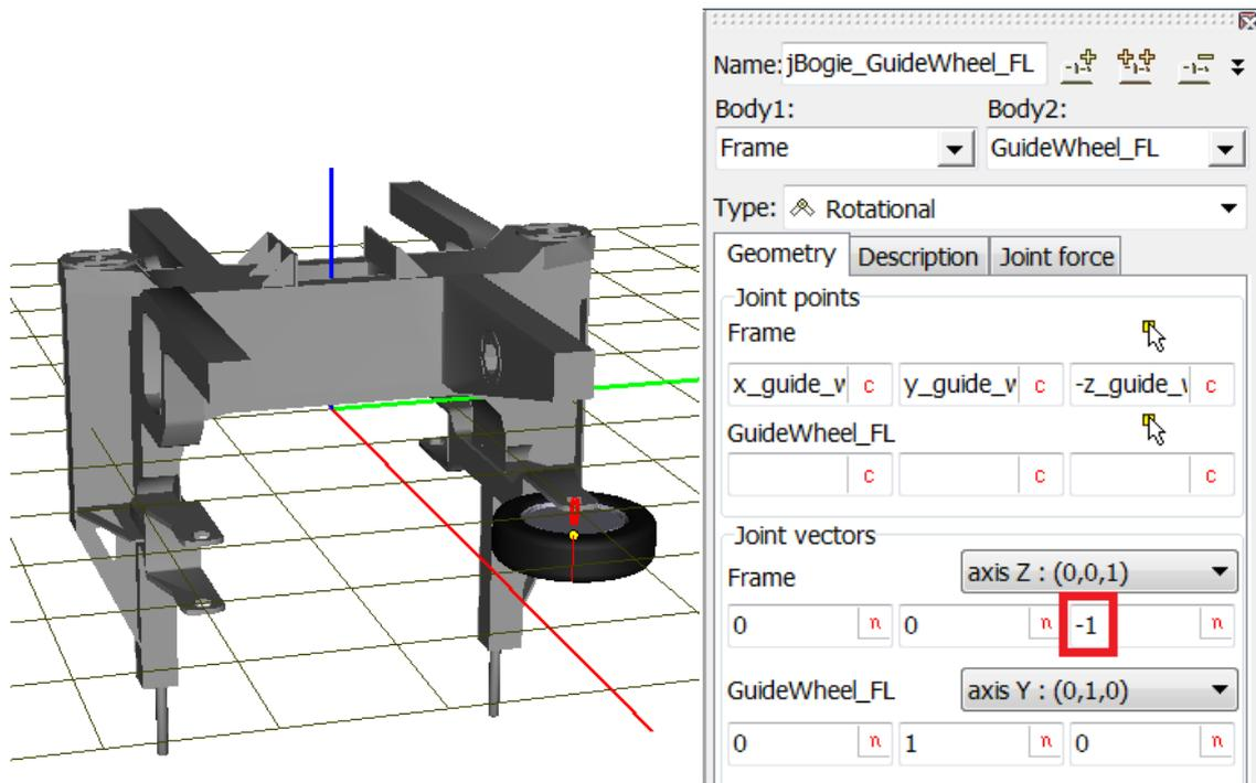
Figure 26.5. Joint for the left guiding wheel
