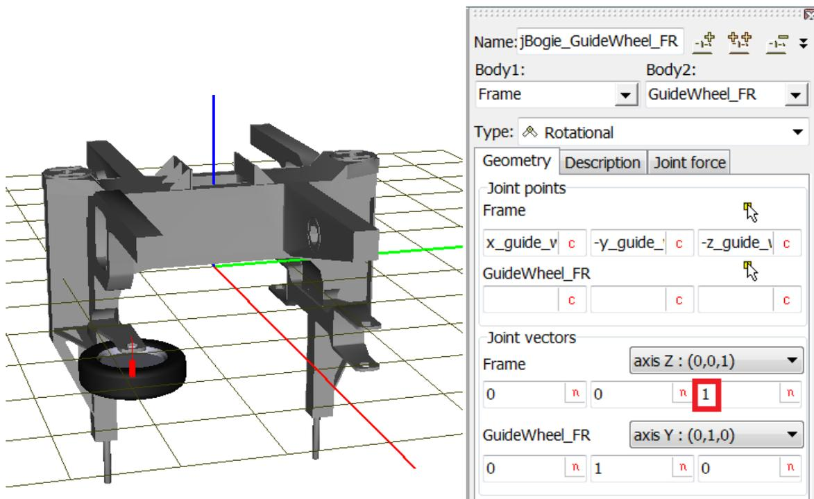
Figure 26.6. Joint for the right guiding wheel
