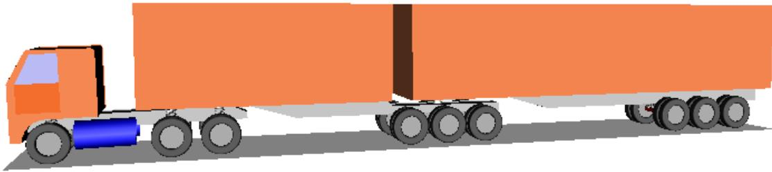
Figure 12.77. 3-unit vehicle: a truck with two semi- trailers
