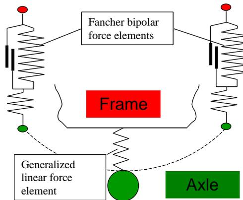
Figure 12.63. Model of a massless leaf spring
