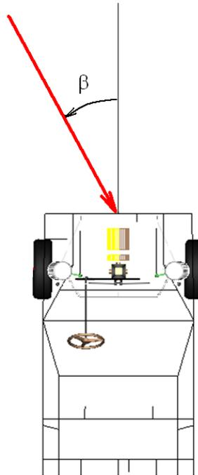
Figure 12.51. Positive angle of relative wind speed direction
