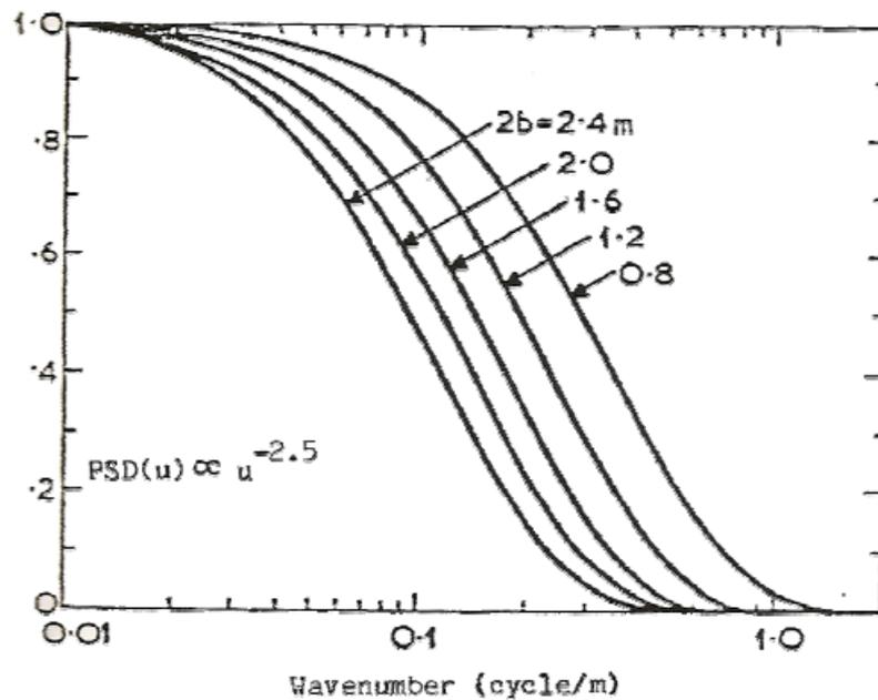
Figure 12.6. Coherence function for different values of track width [3]
