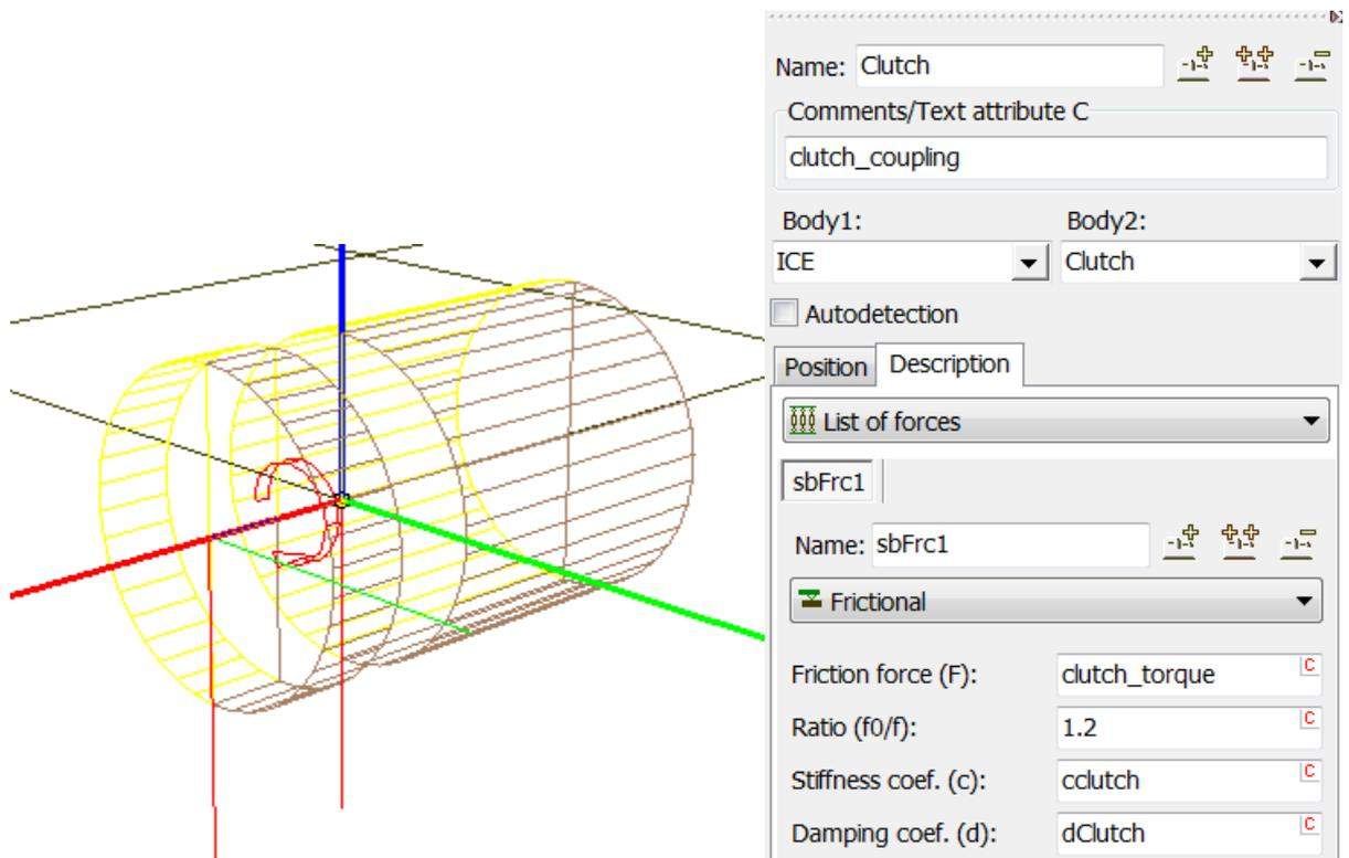
Figure 12.72. Scalar torque modeling friction between crankshaft and second clutch plate
