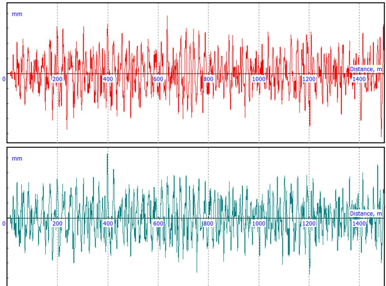
Figure 12.9. Example of road roughness for the left and right tracks
