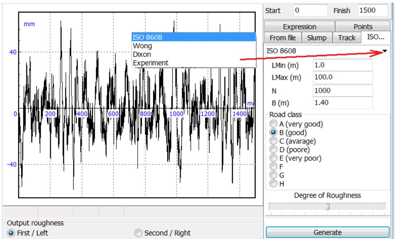
Figure 12.7. Generator of the left and right track roughness
