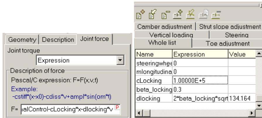
Figure 12.67. Locking joint torque (left); damping constant as an identifier-expression
