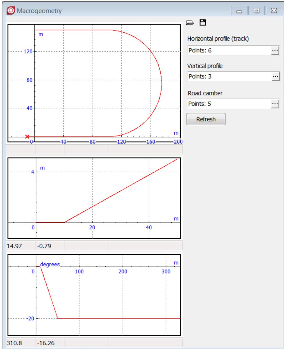
Figure 12.2. Wizard of macro geometry. Horizontal (upper plot), vertical (middle plot) profiles and road camber profile (lower plot)
