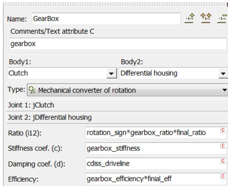
Figure 12.73. Example of modeling gearbox and final drive by single force element
