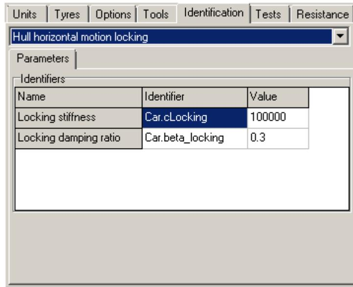
Figure 12.82. Identification of movement locking parameters
