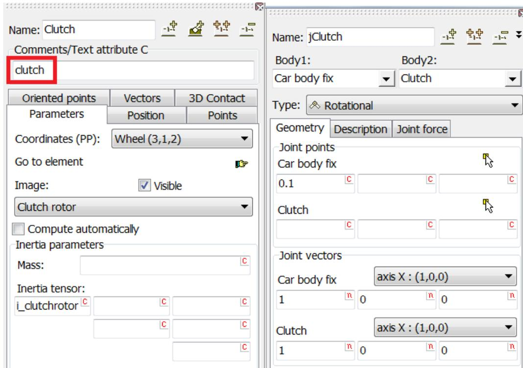
Figure 12.71. Example of a clutch plate as a rigid body and a corresponding rotational joint
