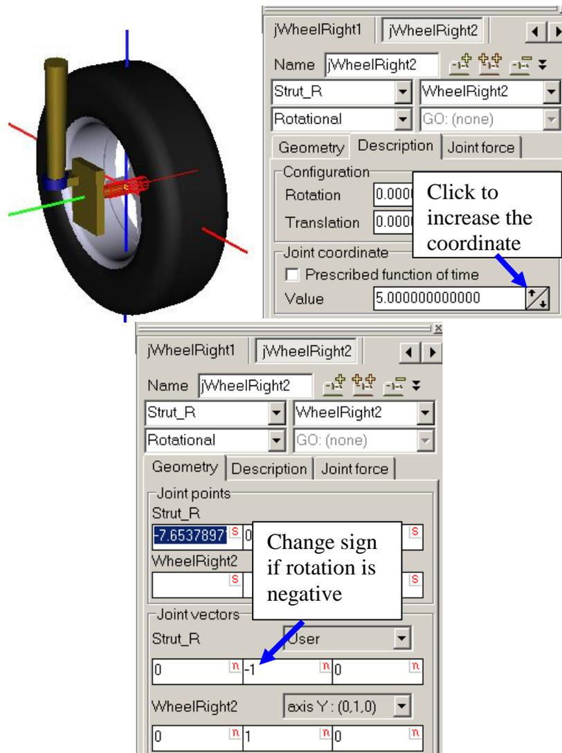
Figure 12.59. Verification of wheel rotational joint
