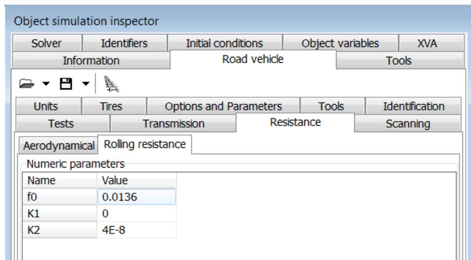
Figure 12.54. Parameters of rolling resistance
