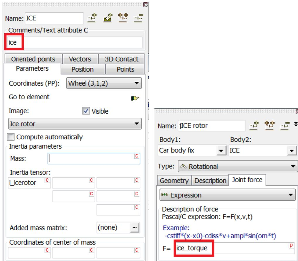
Figure 12.70. Example of an ICE shaft as a rigid body and a corresponding rotational joint
