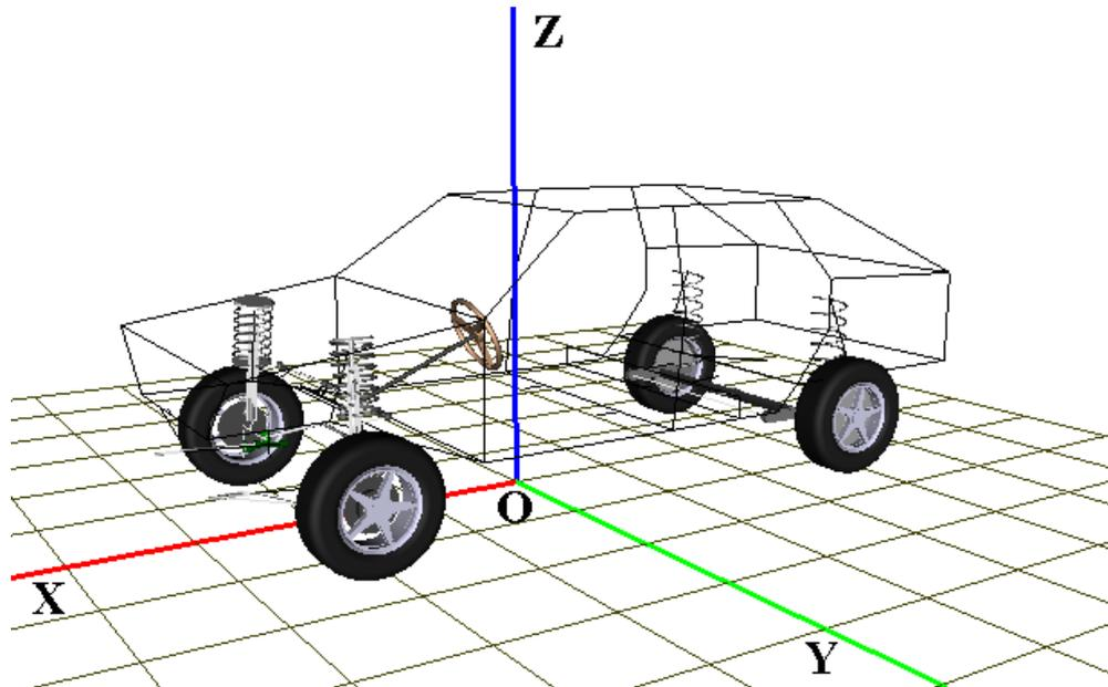
Figure 12.1. Base system of coordinates (SC0)
