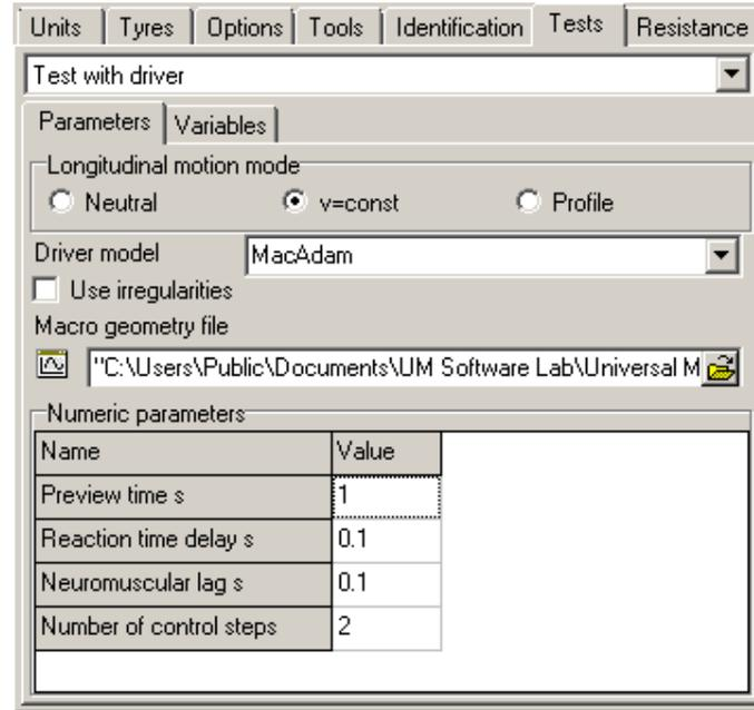
Figure 12.102. Closed loop steering test, MacAdam driver model
