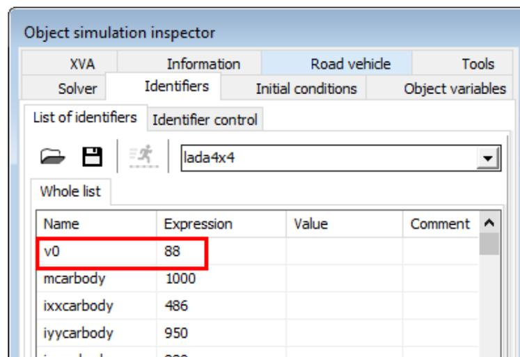
Figure 12.153. Initial speed of the vehicle is 88 km/h
