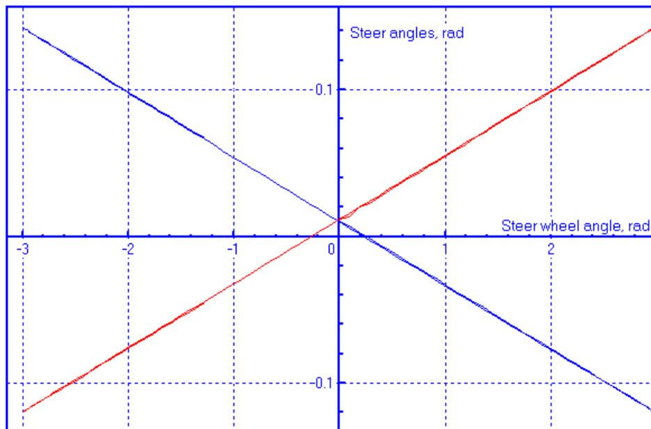
Figure 12.97. Steer angles versus steering wheel rotation angle
