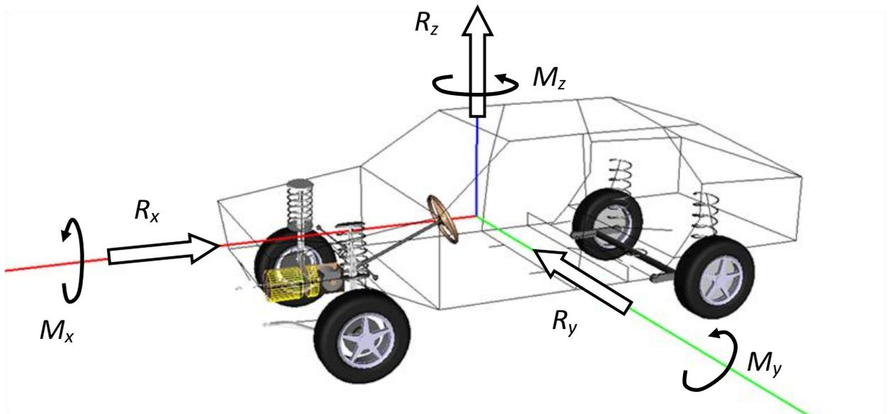
Figure 12.52. Positive directions of aerodynamic forces and moments
