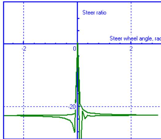
Figure 12.98. Variable  $i_w^e$  versus steering wheel rotation angle
