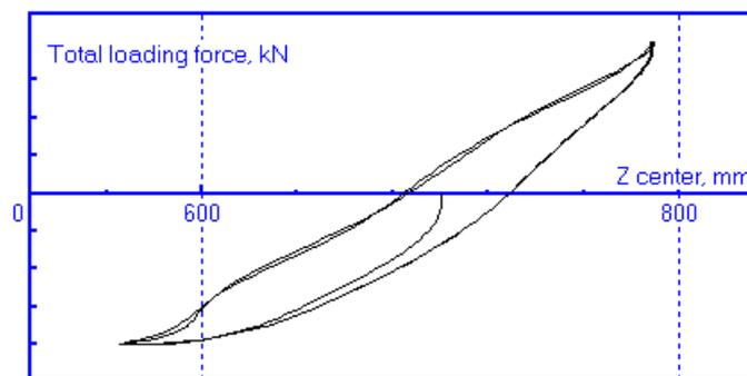
Figure 12.108. Simulation results: Load versus vertical position of center of mass
