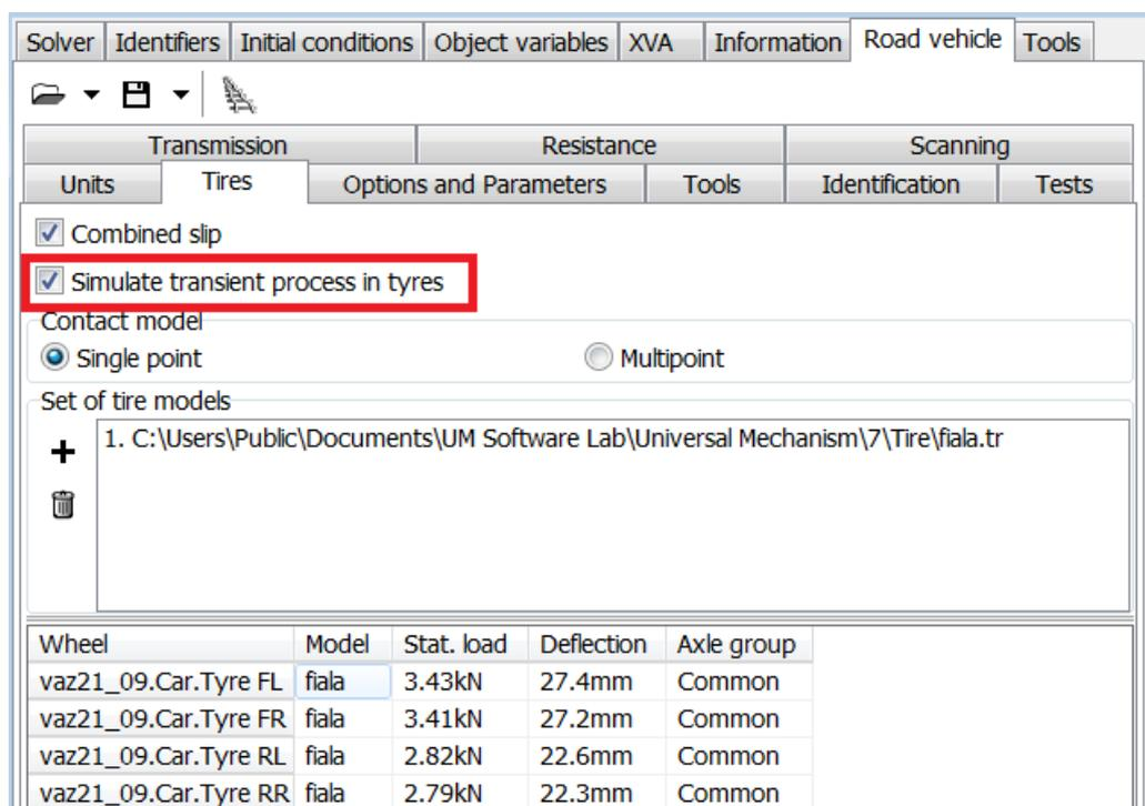
Figure 12.45. Option for transient processes in tire
