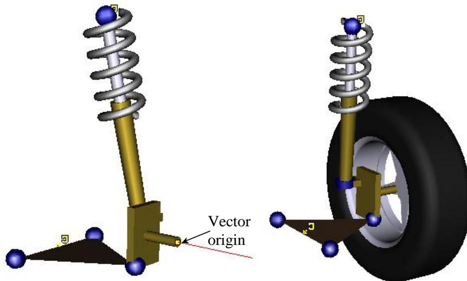
Figure 12.57. Visual adding of wheel and joint
