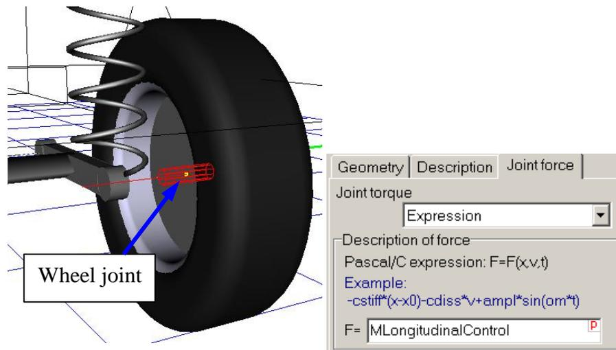
Figure 12.66. Joint torque for longitudinal velocity control
