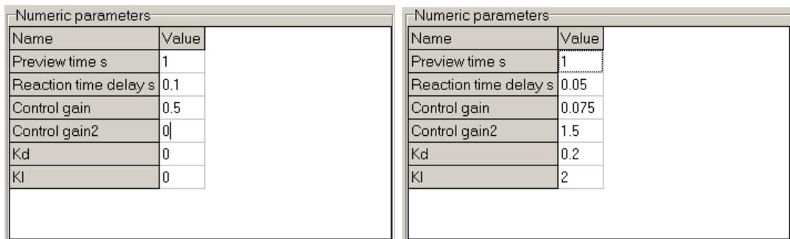
Figure 12.110. Parameters of SOP model (left) and PID-SOP model (right)
