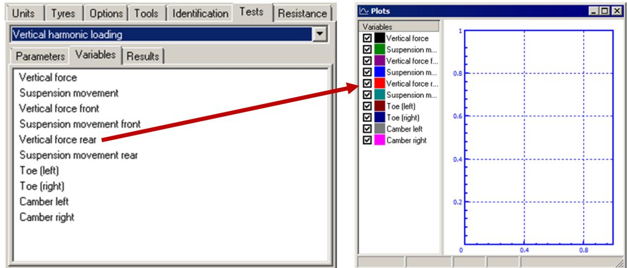
Figure 12.92. Dragging test variables in graphic window
