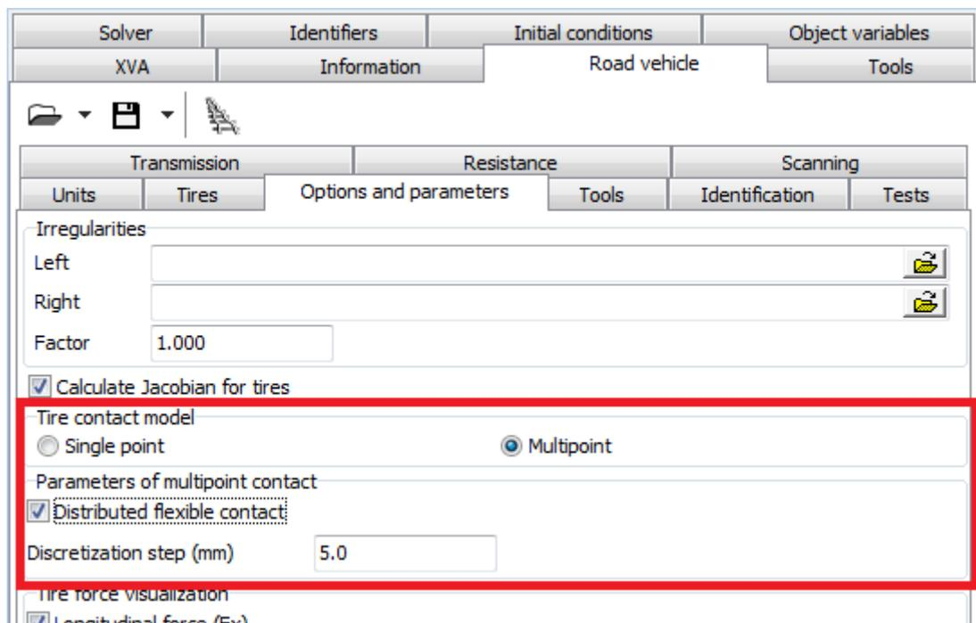
Figure 12.89. Parameters of tire contact model
