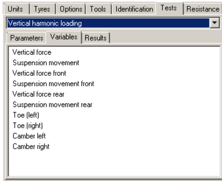
Figure 12.106. Vertical loading test variables
