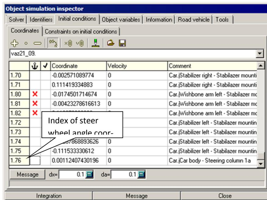
Figure 12.80. Identification of index of steering wheel angle coordinate
