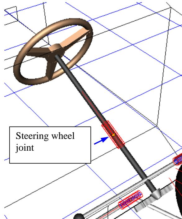
Figure 12.64. Steering wheel joint
