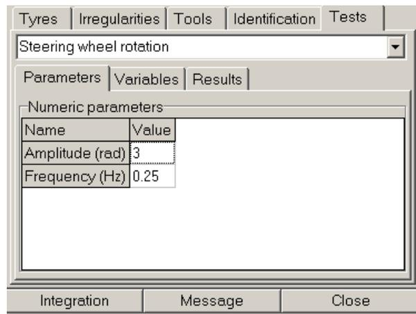
Figure 12.95. Parameters of steering wheel rotation test
